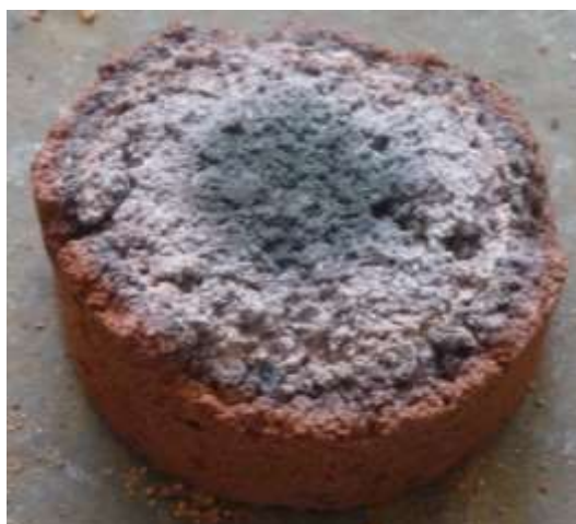
Figure 7: Test specimen with reduced charring on stepped heating
