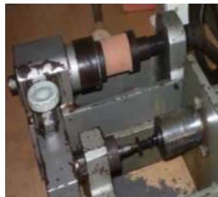
Figure 8: Compression testing with extra load attachment added
