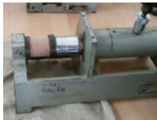
Figure 4: Compression testing on a cylindrical specimen
