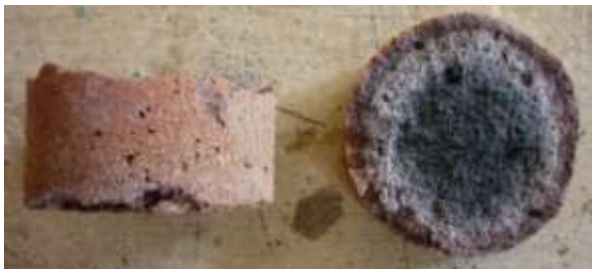
Figure 5: Test specimen with charred core
